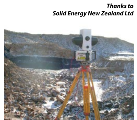
Capturing survey data including location of coal seams in snowy conditions at Stockton Mine
