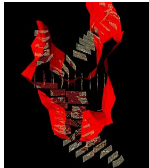
Face mapping sections superimposed on modelled ore zones (red)
