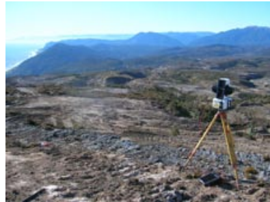
I-Site 4400CR scanner ready for topographic survey in the Stockton open pit
