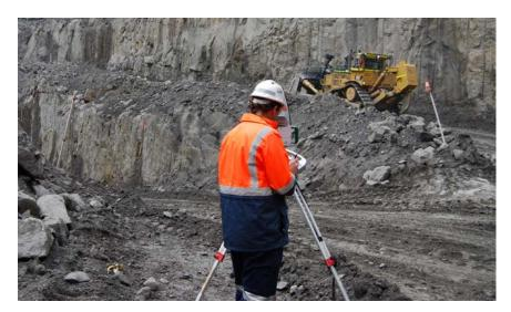
through survey measurement. It is not uncommon for a mine or stockpile surface to now be updated on a daily basis, rather than monthly using conventional survey methods. This higher frequency of measurement will, quite simply, reduce the variance shown in the mining performance from the plan - by enabling better decisions to be made earlier. These laser scanning instruments are now commonly vehicle mounted or automated and can produce millions of 3D data points in a matter of minutes.
