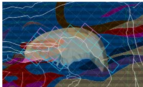
Vulcan 3D mine plan showing scheduled blocks (red = haematite, blue = itabirite)
