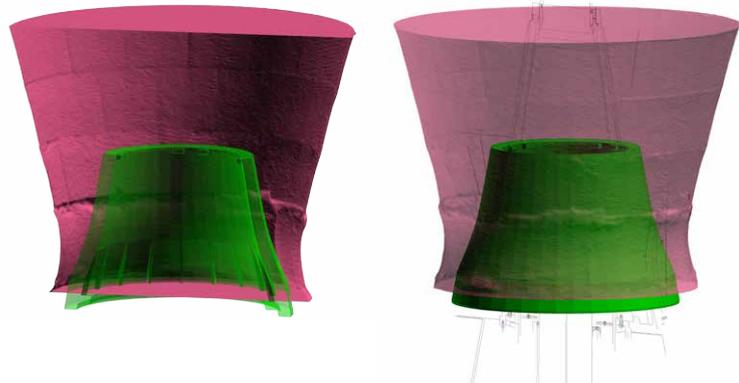
Wide scanning field of view, coarse levelling and 8mm minimum accuracy make the I-Site 8200 system ideal for crusher survey.
