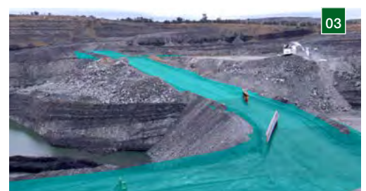
01 Scans are previewed in real time on the tablet 02 Live feedback of scan coverage for efficient survey 03 Design surfaces overlaid on laser scanner images 04 Deformation scan with photograph overlay showing movement and rockfall history
