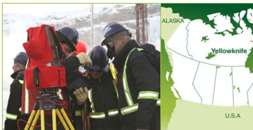
I-Site 4400 scanner with protective jacket to keep out the cold
