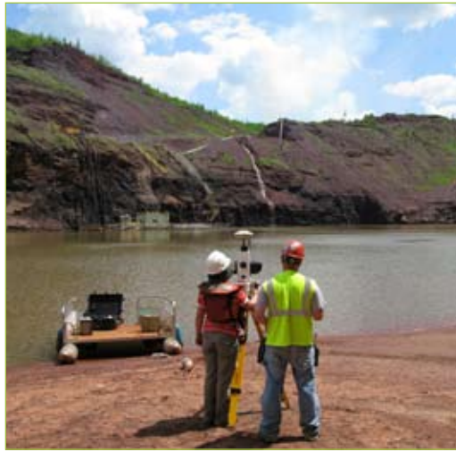
Heather Kutchery, I-Site Technical Consultant and David Oberstar, Hibbing Taconite Surveyor measuring pit walls
