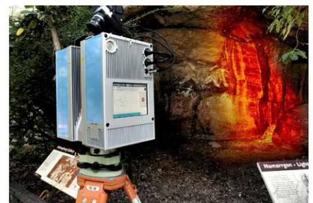
Z+F scanner at the Abangbang Gallery at Nourlangie. The orange coloured area represents a sample of 3D points taken from the scanner.
