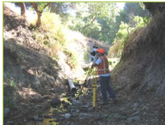
The I-SITE 4400 scanner being used to survey pre-construction project conditions and calculate cut and fill volumes
