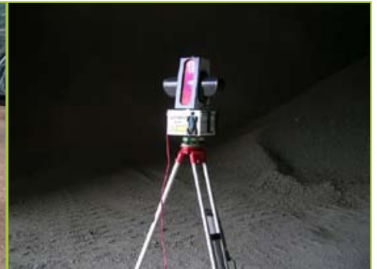
I-Site 4400 scanner inside a clinker shed
