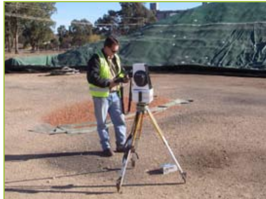
Setting up the I-Site 4400 for stockpile survey
