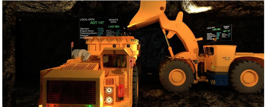
Depending on requirements, individual tags can be provided with virtual ranges; tag settings do not need to be altered, but the on-board equipment associates a specific tag with a particular range.
