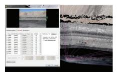
Render high resolution HDR images over 3D scan data for increased accuracy.
