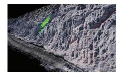
Use Smart Line tools to trace geological boundaries onto high resolution imagery direct from the laser scanner.
