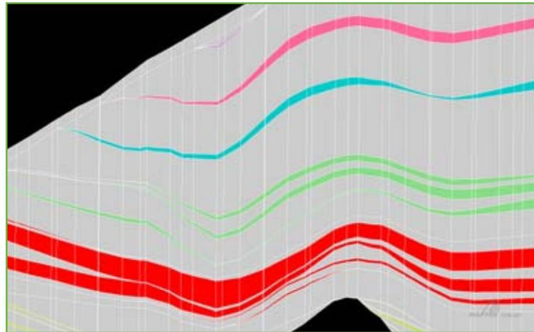
*Cross section through a Vulcan HARP model showing coal seams in coloured blocks with burden shown in grey.*
