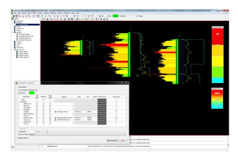
BlastLogic also supports an automated interface with the major drill navigation systems; as-drilled data can be accessed and viewed immediately.
