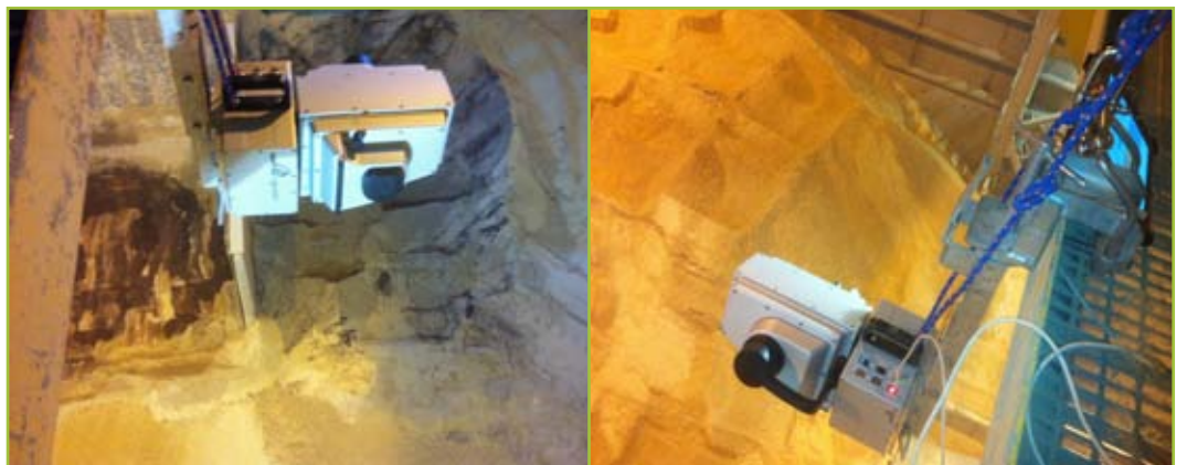
The I-Site 8400 laser scanner mounted on a crane-operated gantry, 12 metres above the stockpile
