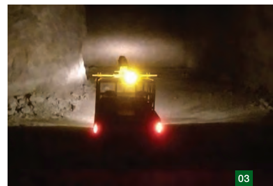
01 Laser scanning setup at drift intersections 02 Modelled surfaces coloured by intensity 03 I-Site 8200 laser scanner mounted on bobcat
