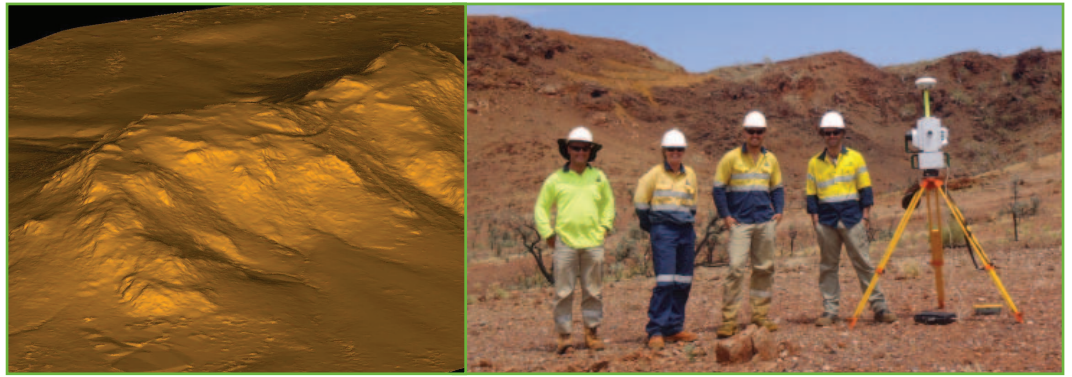
Modelled topographic data for Mount Dove (left) Maptek and Atlas Iron staff with I-Site 8800 laser scanner at Wodgina (right)
