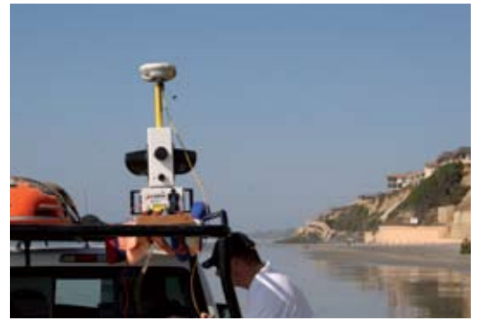
Lifeguard truck moving down the beach during periods of low tide to scan the bluff face
