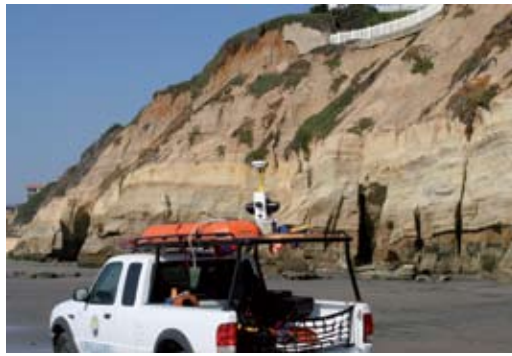
Mounting the scanner on the truck streamlined scanning along the Solana beachfront
