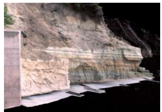
Point cloud of the bluff with beach in the foreground reveals loss of material onto the beach as well as the lithology of the face
