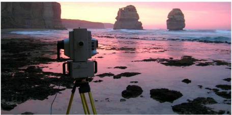
Undercutting causes collapse along the vertical joints resulting in steep slopes along the cliff face. Scanning the area using the Maptek™ I-Site™ 8800 will monitor these undercuts for change.
