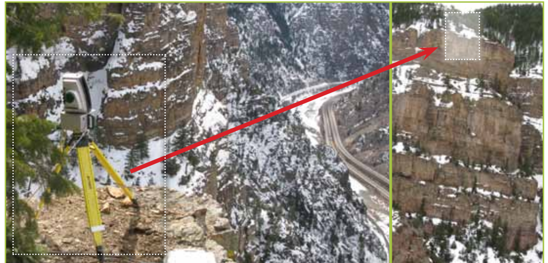
I-Site 8800 laser scanner overlooking rockslide with the arrow pointing to the position of scanner on canyon wall rim
