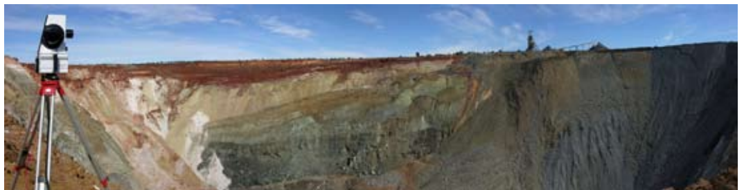
Second set up at end of ramp cut off by wall failure
