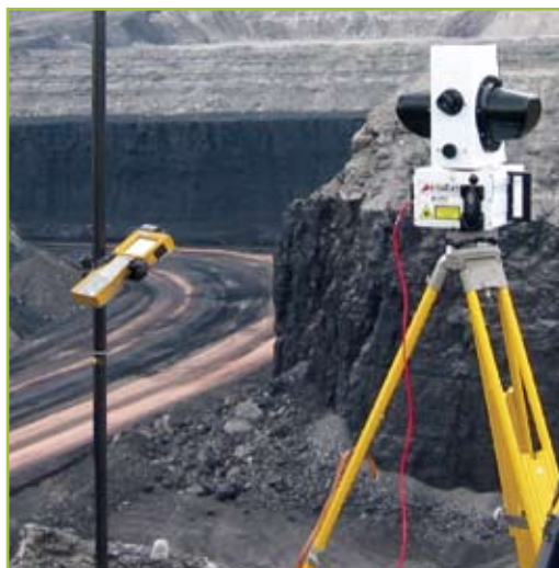
I-Site 4400 scanner and GPS setup at Peabody's North Antelope Rochelle mine
