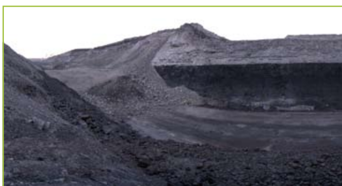
Panoramic image of a cast blast, captured simultaneously with scans using the I-Site 4400 integrated high resolution digital camera
