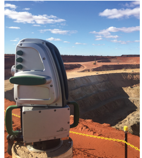
XR3 laser scanner set up on pillar to scan pit surface
