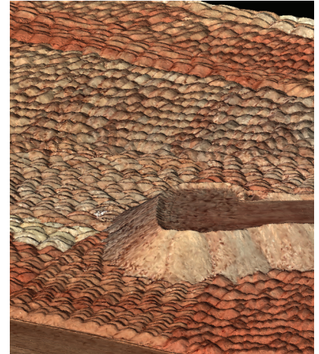
UAV captured waste dump surface in PointStudio
