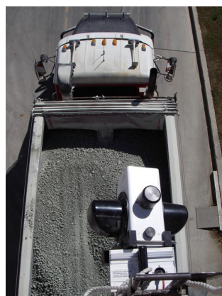
I-SITE scanner (left) measuring truck loads, and resultant modelled scan data (above)
