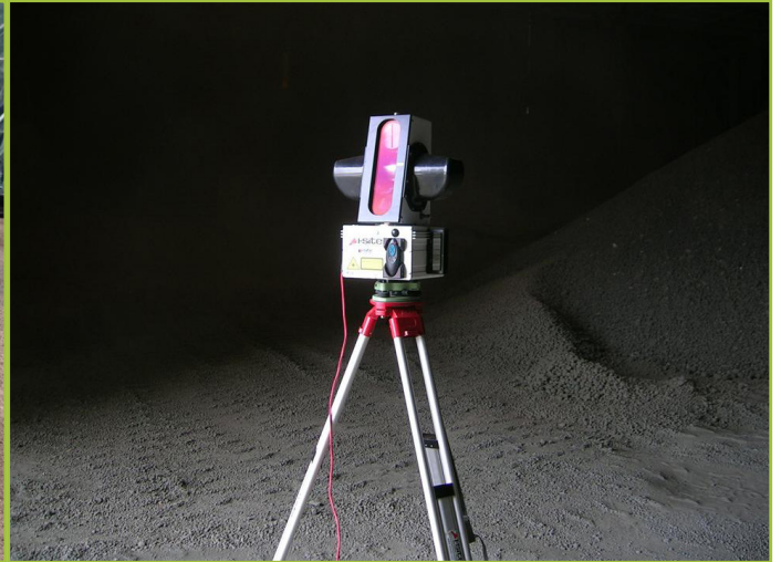
I-Site 4400 scanner inside a clinker shed
