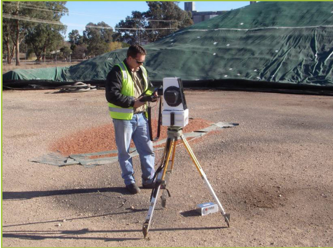
Setting up the I-Site 4400 for stockpile survey
