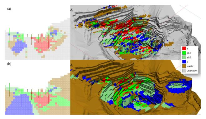
**Figure 4.** Cross section (left) and 3D view (right) of conventional method (**a**), and DomainMCF predictions (**b**). ID2 estimates were limited by a search ellipsoid while DomainMCF was free to estimate the entire block model.
