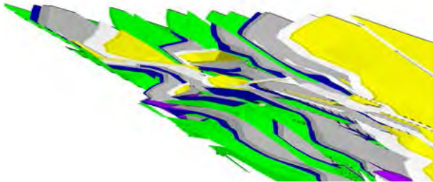
Isometric view of the steeply dipping multi-seam structurally complex deposit
