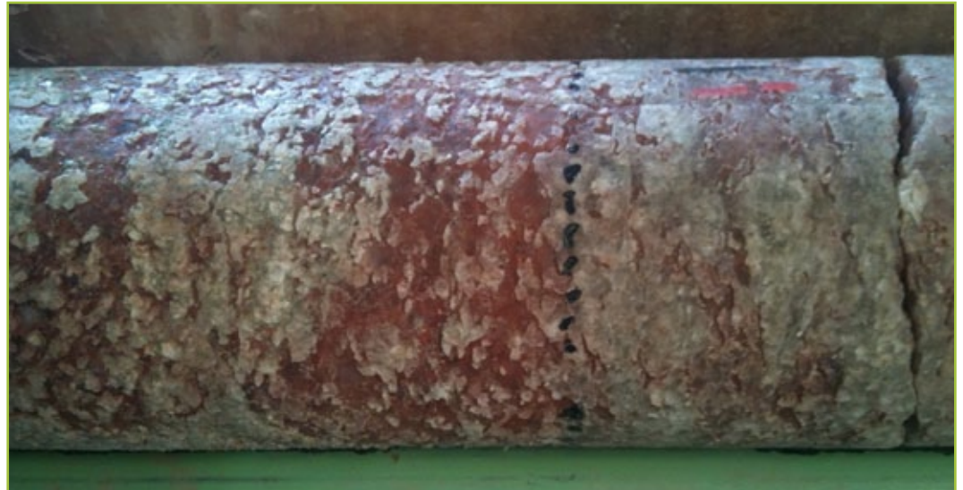
The drill core shows clearly distinguishable strata, KCl salt crystals, areas of impurity and indicator clay horizons
