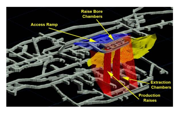
Having pioneered a unique raise bore mining method for uranium production, Cameco uses Maptek Vulcan™ for planning and production as well as critical geotechnical modelling.
