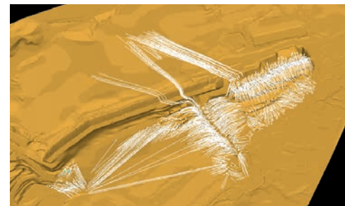
Rolling natural final landforms generated in 3d-DigPlus (above) and push distance arcs indicating material movement directions (below)
