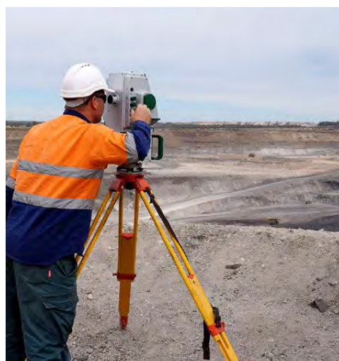
The new I-Site 8820 laser scanner has a range of 2000 metres
