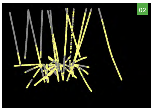
Location of (L) Poor-Fair RMR and (R) Fair-Very Good RMR highlighted in yellow
