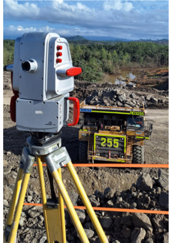
PointStudio filtering and processing tools streamline the generation of capacity volumes after haulage trucks are scanned by the long range LR3 laser scanner (right)
