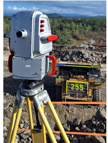
PointStudio filtering and processing tools streamline the generation of capacity volumes after haulage trucks are scanned by the long range LR3 laser scanner (right)
