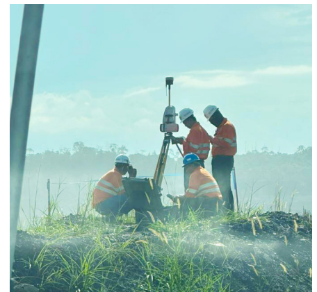
Maptek laser scanning technology helps the Thiess survey division to safely collect data without interrupting operations and to generate accurate mapping and survey deliverables
